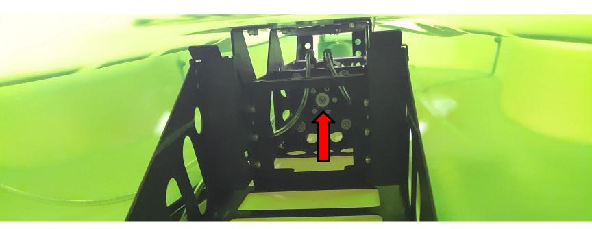
With the **board standing upright** on its tail, open the front main hatch and looking down inside the board, you will see the back of the motor.
