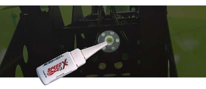
Then apply lubrication to the perimeter of the center bolt. We suggest Corrosion-X 77001 Available on Amazon For best results. The board should remain standing for at least 4 hours to allow the lubricant to penetrate down though the bearings in the core of the motor. Remember, with the battery out always verify the drive line turns freely before use.
